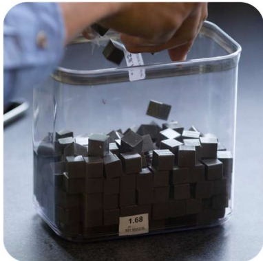
MatchPRO RFID density tracers.
