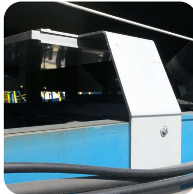
Detector installed under product conveyor.
